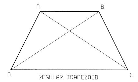
THE DIAGONALS ON ANY SQUARE, RECTANGLE, OR REGULAR TRAPEZOID ARE ALWAYS EQUAL. "AC"="BD" IN EACH FIGURE ABOVE. THIS PRINCIPLE CAN BE APPLIED WHEN TRYING TO SQUARE FLATS, DECKS OR OTHER SCENERY.
