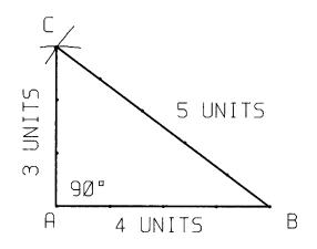
(NOTE: THIS IS NOT A 30°-60°-90° TRIANGLE. ANGLE "B" IS NOT 30° AND ANGLE "C" IS NOT 60°)
